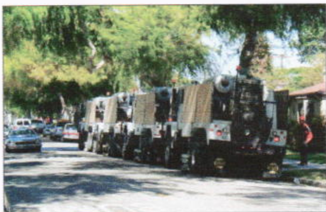
A public demonstration was held in Culver City for city council members and other interested parties. Surveying operations were conducted on the street on which the city's mayor lives, and included monitoring vibration and noise levels inside the mayor's house.
